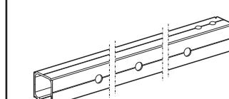
1 running rail pre-drilled, 2000 mm
